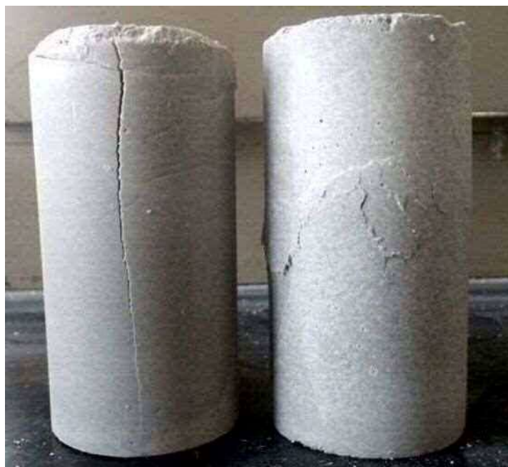
Fig. 6-31 供試体の破壊状況 (左 : B5P0, 右 : B5P2) The destruction situation of the test piece (left: B5P0, right: B5P2)
